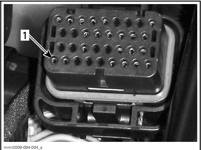
1. Terminal fully inserted in connector
